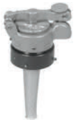
FA-1D Lockable Flame Arrestor Fuel Cap 043947 Field Fuel cap can be padlocked to prevent vandalism. A built-in flame arrestor prevents flames or sparks from entering the fuel tank.
